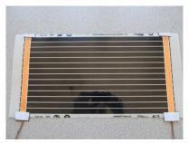
1. For easier understanding only one section of the carbon film is shown. That's how it should look when read (ph1). On one side the cold ends which are used for the wiring are mounted, on the other side it is covered with safety tape on top of the copper stripe.
