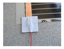
5. On the back side the copper stripe is insulated for safety with the special tape - ph6 and ph7.
