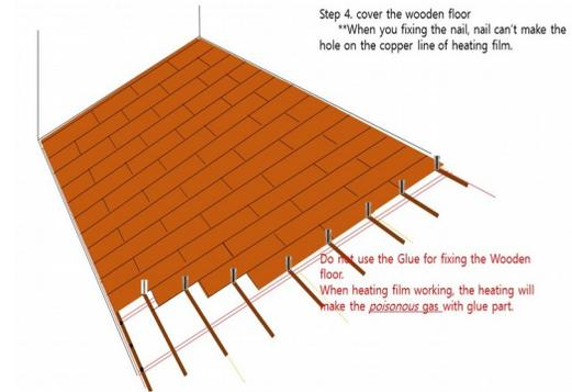
A special installation of the carbon heating film. It is used for nailed wooden floors.
